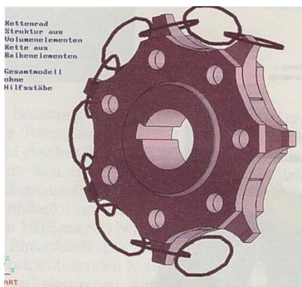
1: Modelling of the system chain / chain sprocket
