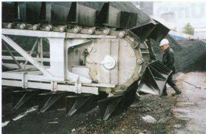
The noise level generated by this equipment is well below the allowed values thanks to the self-adjusting chain sprockets.
