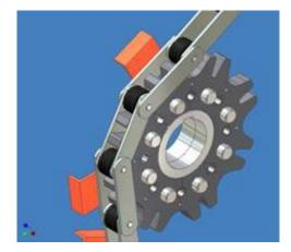
This means that **all the teeth of the** sprocket are **equally loaded by** the selfadjusting sprocket I invented. This leads to the fact that the chain, which is manufactured depending upon size with a **very high financial and labor expenditure,** whereby naturally **high energy costs result**, substantially longer lasts, since it is not so strongly loaded by the movable teeth of the chain wheel.
